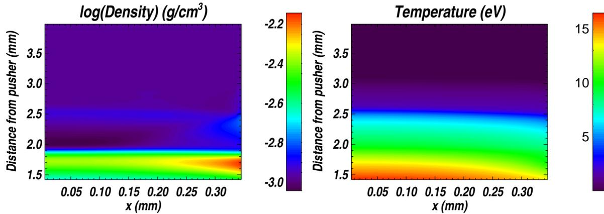
Fig. 2. Maps of density (left) and temperature (right) of a 2D axisymmetric simulation performed by HERACLES with a wall transmission of 60%.
