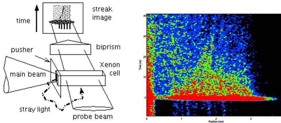
**Fig. 1.** Left: Schematic experimental setup. Right: false color image of the streak camera recording. The shock propagates from the left to the right. The horizontal bright spot occurs during the laser pulse, 10 ns after the beginning of the record. The initial position of the piston is on the left.
