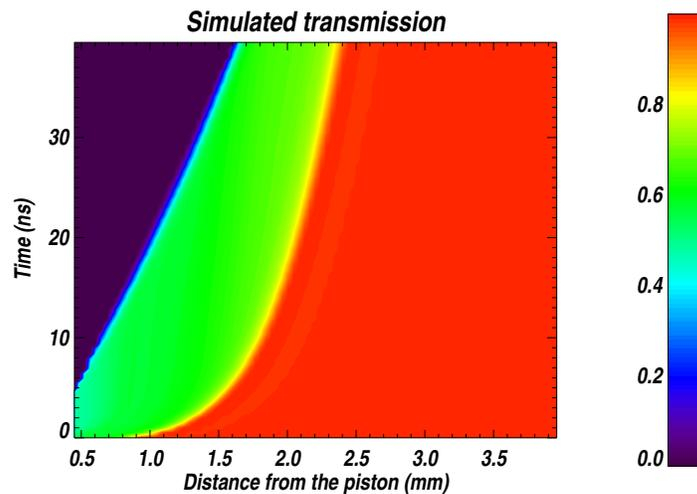
**Fig. 5.** Simulated transmission of the cell using the HERACLES simulation
