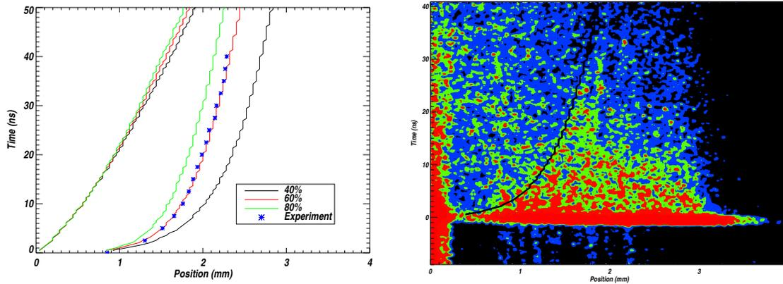
**Fig. 4.** Left: positions of the shock and the precursor versus time for different values of wall transmission. Right: the precursor position obtained with HERACLES compared to the experimental data.
