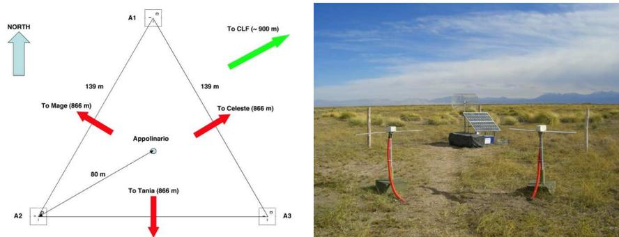
**Fig. 1. Left :** Global setup of the RAuger experiment. The 3 stations, namely A1, A2 and A3, are around the additional tank named Appollinario at the center of an elementary triangle of the Auger surface detector (not on the figure). The Central PC is at the CLF, 900 m away. **Right:** Detail of one of the 3 radio stations. The 2 short active dipoles (EW and NS) are at the foreground. The electronic box, solar panels and the WIFI antenna for data transmission are just behind.
