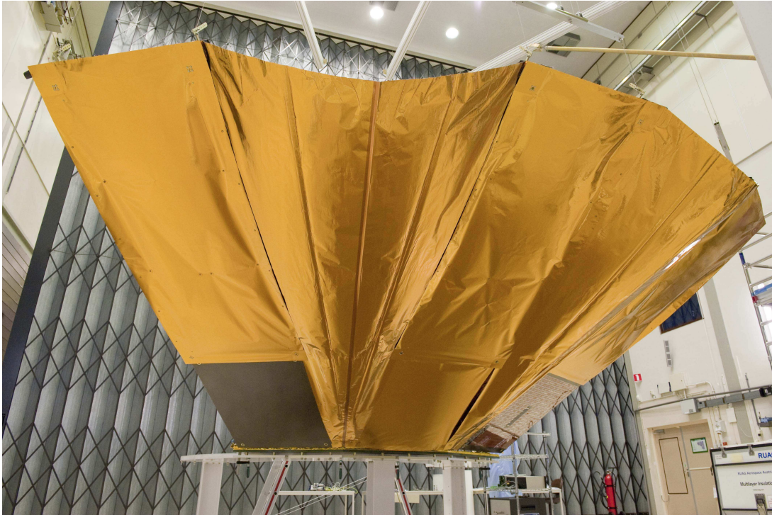
Fig. 1. This picture shows the Gaia deployable sunshield assembly (DSA) qualification model (QM) during deployment tests in the cleanroom at ESTEC, Noordwijk, The Netherlands. This model arrived at the ESTEC test facilities on 29 June 2009 for thermal tests inside the Large Space Simulator (LSS). Before the tests inside the LSS, several deployment tests of the sunshield were performed in the cleanroom at ambient conditions. This view shows the qualification-model sunshield during this deployment. The gold-coloured blanket of multi-layer insulation (MLI) is the sun-side blanket of the sunshield. Like the parallel-installed, shadow-side blanket behind it, it is made up of fixed sections attached to the three rectangular frames, and two foldable sections between the frames which are rolled in stowed configuration and unroll during deployment. The dark-coloured squares at the left and right bottom of the sunshield are solar panels. Copyright: ESA.
