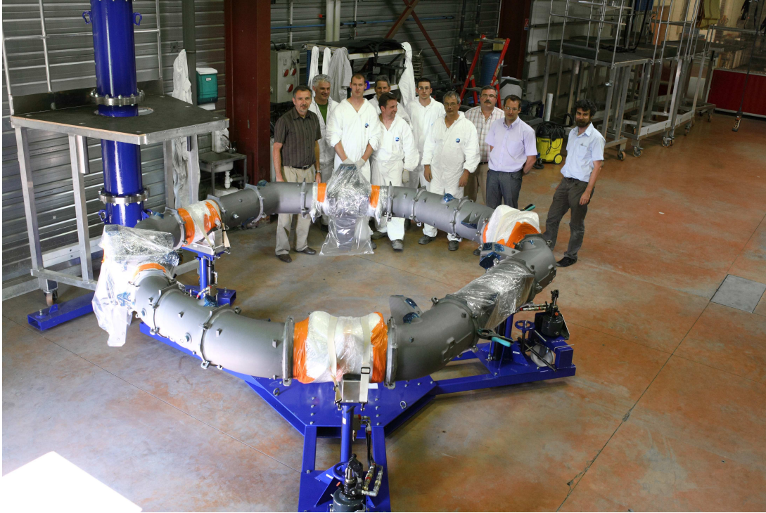
Fig. 2. This picture shows the Gaia flight-model torus at the BOOSTEC premises at Bazet, near Tarbes, France. Pictured are members of the BOOSTEC and EADS Astrium SAS team just after the torus removal from the brazing furnace. The 3-metre-diameter, quasi-octagonal torus, which will support the two Gaia telescopes and the focal-plane assembly (FPA), is composed of 17 individual, custom-built, Silicon-Carbide (SiC) segments, all of which were constructed by BOOSTEC under contract to the Gaia prime contractor, EADS Astrium SAS. Starting on 28 April 2009, the 17 elements were assembled and aligned into the form of the torus. The torus brazing took place from 24–29 June 2009. Following the successful completion of the brazing, the torus has been delivered to EADS Astrium SAS in Toulouse for assembly of the bipod and release mechanisms (BRMs). Copyright: ESA.
