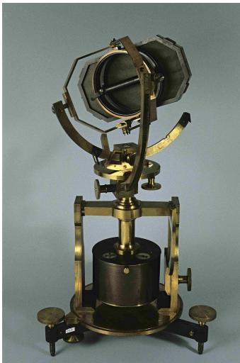
Fig. 7. Heliostat of Silbermann type, built by Duboscq in 1883, Cliché M. Dubau©inventaire général ADAGP.
