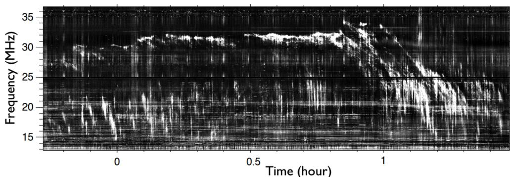
**Fig. 3.** Dynamic spectrum of Jupiter’s decameter emission observed by a single LSS antenna with GURT preamplifier, on 9 oct. 2011. Jupiter bursts, inclined in the displayed time-frequency plane, have an intensity of a few % of the galactic background (the latter has been subtracted in the displayed dynamic spectrum). They are clearly detected down to 13–14 MHz.
