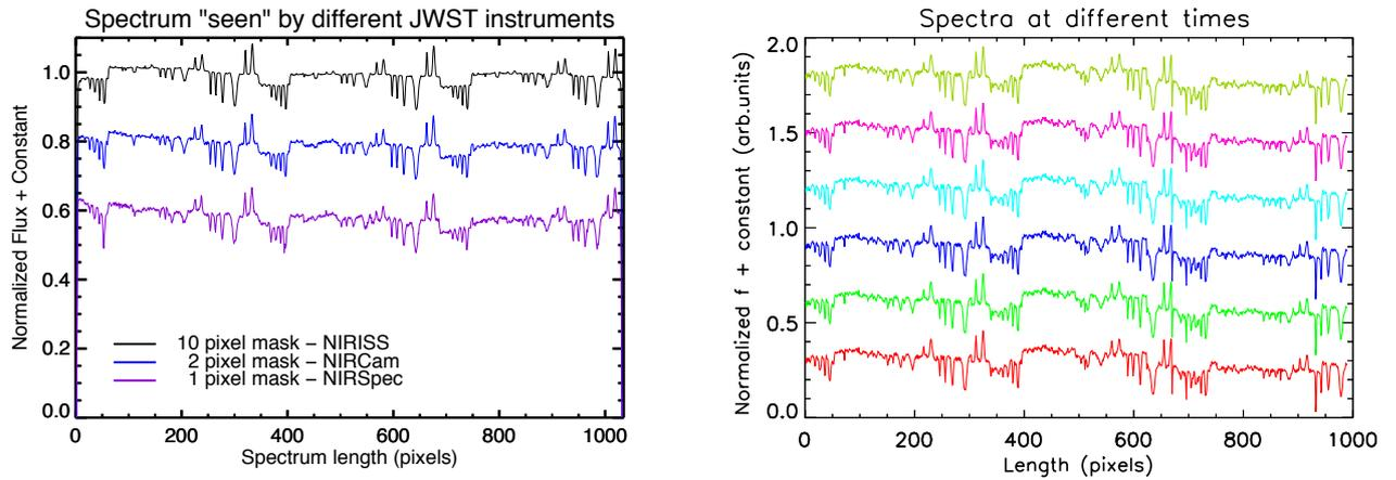
**Fig. 1. Left:** The detected spectrum, emulated by the three different masks which correspond respectively to the three following JWST instruments: NIRISS, NIRCam, NIRSpec. **Right:** Six of the synthetic spectra, produced by the 10-pixel width mask, at different times (shifted for clarity). The spectrum length is 1000 pixels. The features represent emission and absorption lines. After decorrelation of vertical and lateral offsets we achieve a precision  $<30$  ppm.
