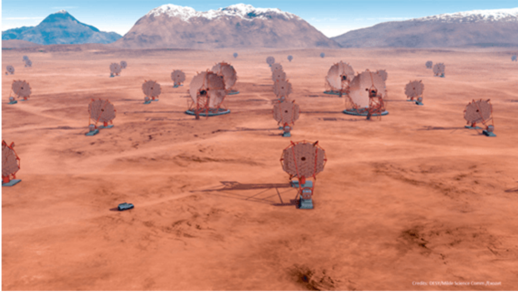
Fig. 4. Artist's view of the future southern Cherenkov Telescope Array. Telescopes of different types and sizes allow to cover a very large domain in energy, from 20 GeV to 300 TeV.
