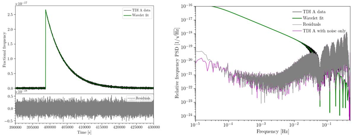
**Fig. 3. Left:** Result of the time-domain estimation using a sparse wavelet model. The top panel represents the observed data (black) and result of the fit (green) and the bottom panel represents the fit residuals. **Right:** The same data is plotted in the frequency domain, along with the same data with the stochastic noise only (magenta) for comparison.
