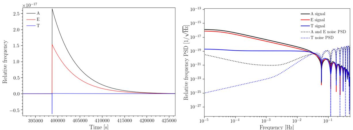
**Fig. 2. Left:** Time-domain simulation of a LPF-like glitch TDI signal for channels A, E and T. **Right:** Periodogram of the TDI simulation in the frequency domain. The glitch spectra are represented by the solid lines, while the LISA noise sensitivity is represented by the black dotted line for channels A and E, and by the blue dotted line for channel T.
