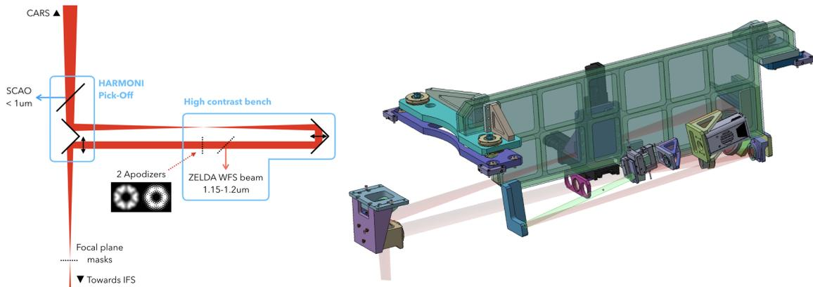
**Fig. 2.** Conceptual view (left) and 3D rendering (right) of the HC subsystem of HARMONI. Light is picked right after the SCAO dichroic and sent towards the HC bench where it is optically processed before being returned towards the IFS. The front facing optics are those of the Zernike wavefront sensor.
