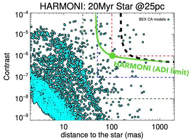
**Fig. 1.** Contrast separation diagram showing a simulated population of young giant planets around 25pc stars based on the Bern model (Mordasini 2014). The dashed black line represents the contrast limit of VLT-SPHERE, while the solid green line does the same for HARMONI, assuming an ADI-based post-processing of the data.
