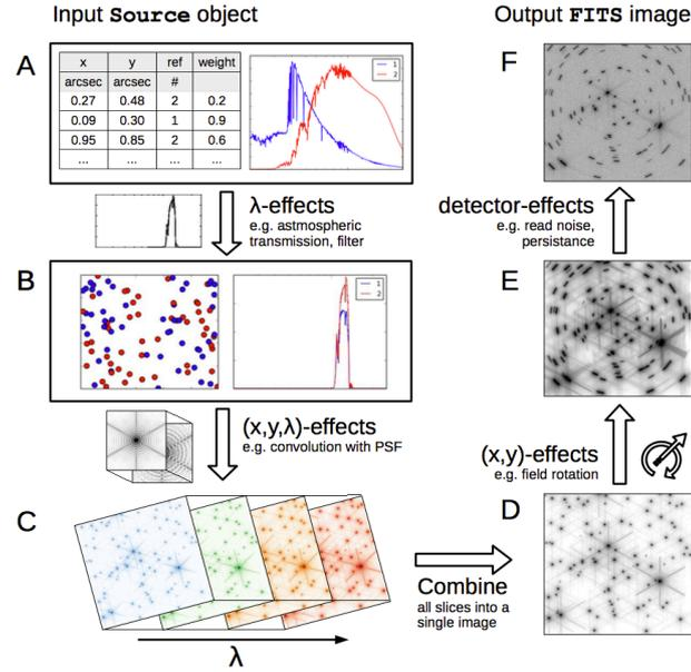
**Fig. 3.** SimCADO data model, representing the flow of events from the creation of the source object (here a mock open cluster) to the output FITS image. More details in Leschinski et al. (2016)
