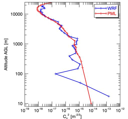
**Fig. 2.** Median profiles of  $C_n^2$  on 2018/08/27
