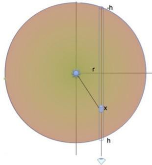
**Fig. 3.** Sketch of the adopted geometry for the radiative transfer model
