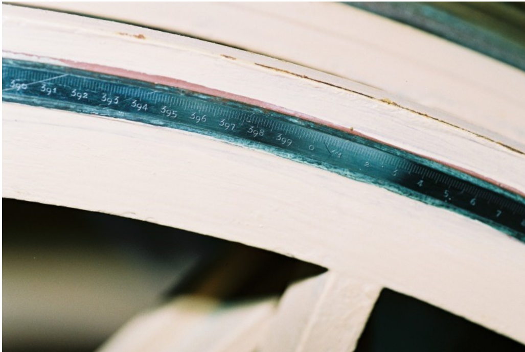
Fig. 3. Meridian telescope's circle graduated from 0 to 400 grads
