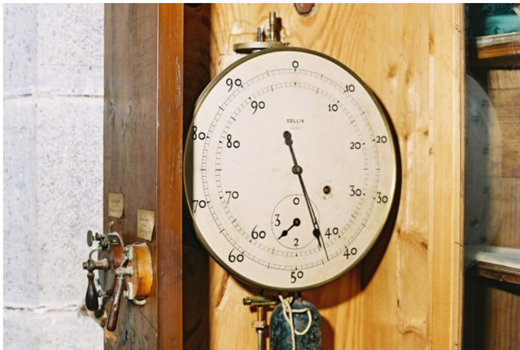
Fig. 2. Decimal clock with 100 "minutes", 100 "seconds" and 4 quarters of a day (or "quadrants").
