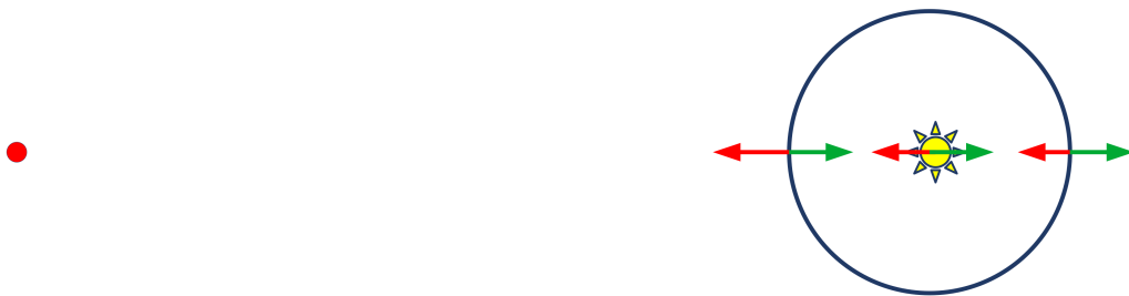
Fig. 1. Tidal acceleration in the star-centered frame. Red arrows to the left: direct force from the planet (red dot). Green arrows to the right: indirect term.
