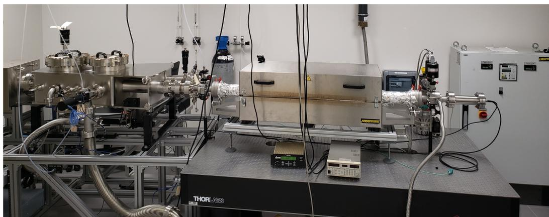
**Fig. 2.** VUV platform developed at LISA for absorption cross section measurements.
