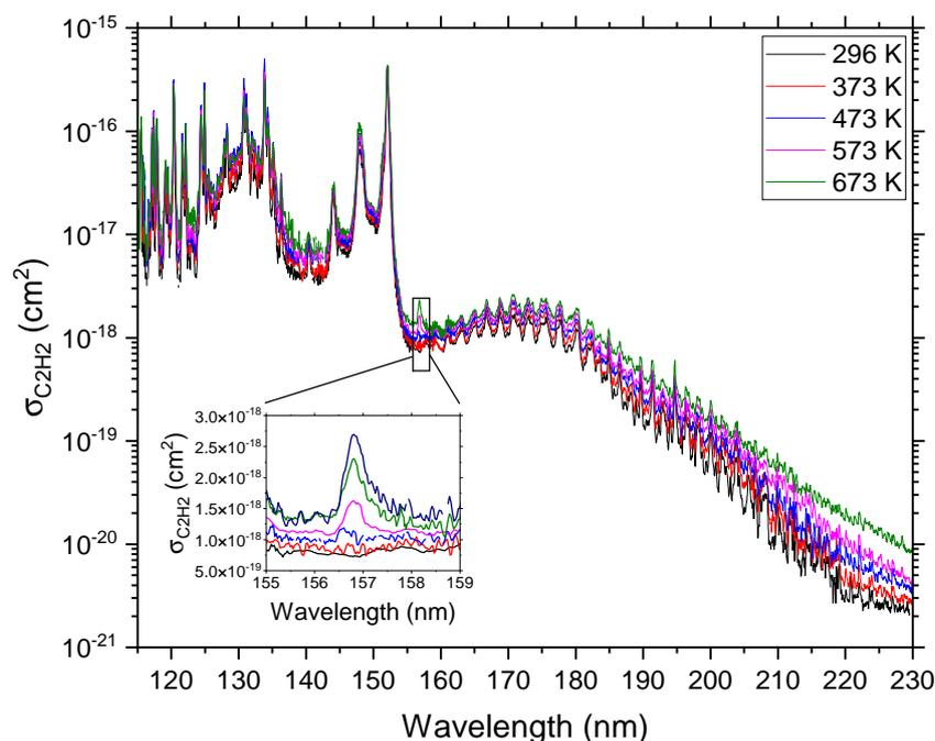
**Fig. 1.** Evolution of the absolute absorption cross section of  $C_2H_2$  as a function of the temperature. Spectra were measured from 115 to 230 nm at LISA with an instrumental resolution of 0.046 nm.
