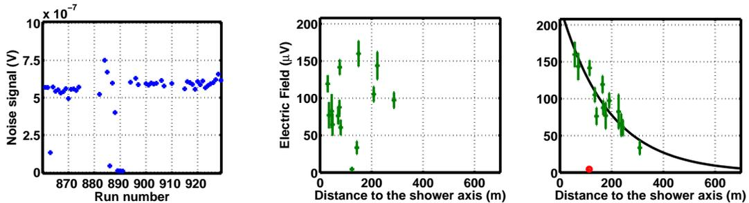
**Fig. 3.** **Left** : The monitoring shows a breakdown, between the 875th and 895th run (one month) for one antenna. **Center** The result of the lateral distribution fit for one unexpected profile, during the antenna breakdown. **Right** : Result after the removing of the dysfunctional antenna (red dot at the bottom) during the minimization process of the  $\chi^2$ . An exponential profile is recovered. Consequently, the location of the shower core can change.
