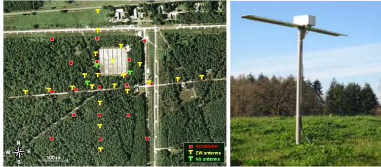
**Fig. 1.** **Left** : Schematic aerial view of the Codalema experiment. Plastic scintillators are depicted as squares, antennas as T, oriented in the NS and EW direction. **Right**: One dipole of the antenna array.
