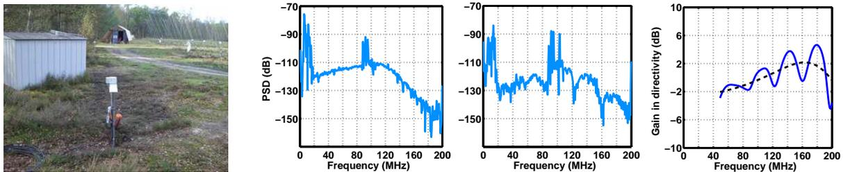
**Fig. 4.** From left to right **A** : Antenna close to the metallic shelter. **B** : Raw spectrum of a powerful event seen by one normal antenna. **C** : Raw spectrum of the same event seen by the antenna close to the metallic shelter. **D** : Simulated gain vs frequency for two antennas, for a white noise in the arrival direction of the cosmic ray (without considering the amplifier response). Dotted lines : without shelter. Solid line : with the metallic shelter.
