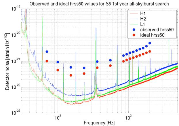
**Fig. 2.** Plotted are the noise floors of the three LIGO detectors, with overlaid the expected from gaussian noise (in red) and actual 50% sensitivity to GW (in blue).
