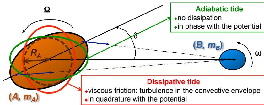
**Fig. 1.** Tidal interactions in a binary system. Body B exerts a tidal force on body A, which adjusts itself with a phase lag  $\delta$ , because of internal friction. This adjustment may be split in an adiabatic component, which is in phase with the tide, and a dissipative one, which is in quadrature.
