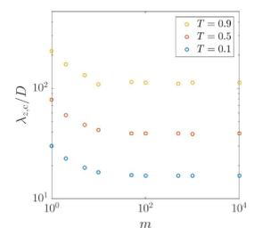
**Fig. 2:** Vertical cut-off wavelength as a function of number of steps, measured for 3 criteria on  $T$ .
