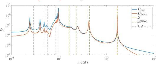
**Fig. 3:** Viscous (blue), and thermal (red) dissipation rates as a function of forcing frequency  $\omega/2\Omega$ . Each resonant peak corresponds to the excitation of a free mode of the staircase (see 2).
