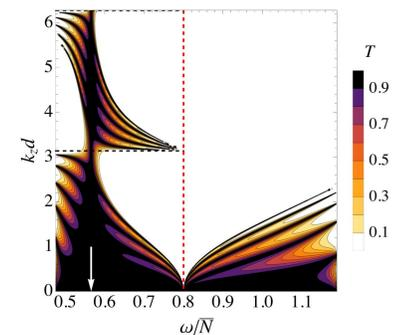
**Fig. 1:** Transmission coefficient as a function of wave's frequency and vertical wave number. White arrow:  $\omega = 2\Omega\cos\theta$ , dashed red line:  $\omega = 2\Omega$ . Each band of perfect transmission corresponds to a free mode of the staircase.
