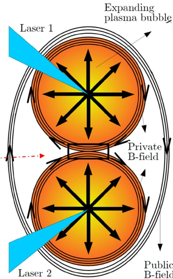
Focusing a high-power laser onto a solid target generates a plasma bubble with a megaGauss scale magnetic field
