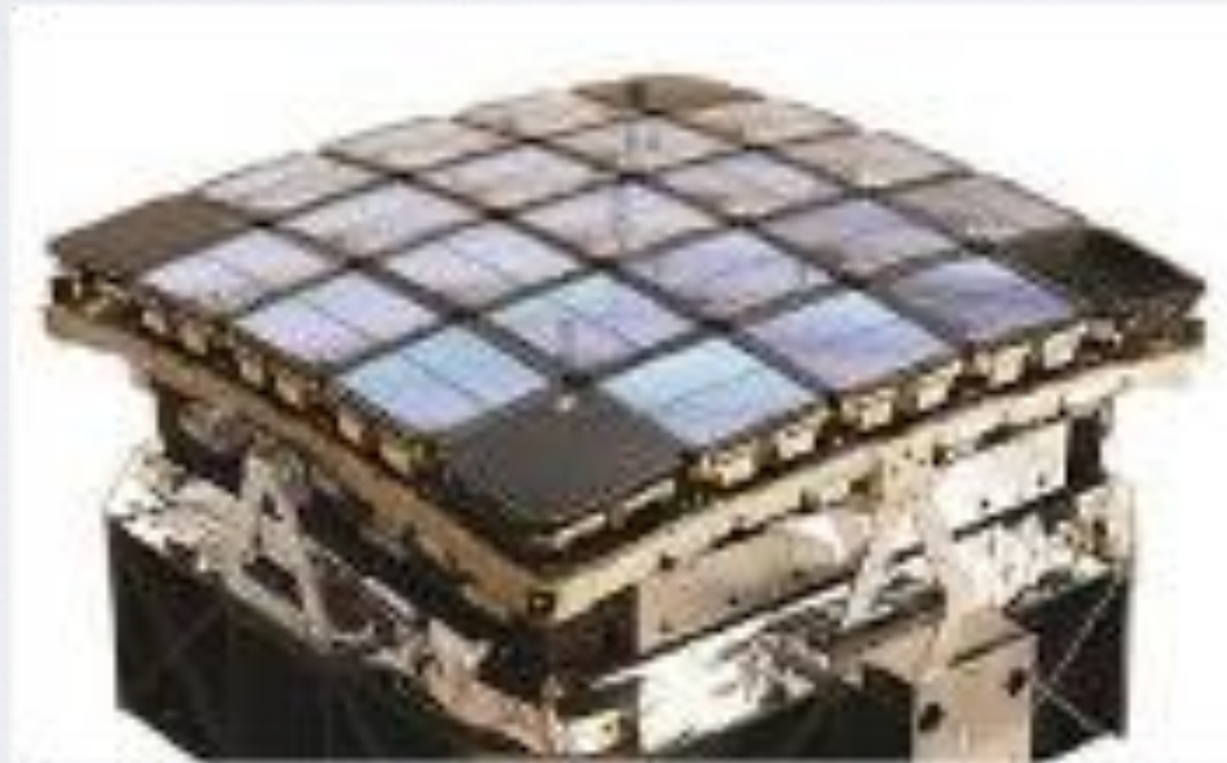
Kepler focal plane, 42 flat CCDs
