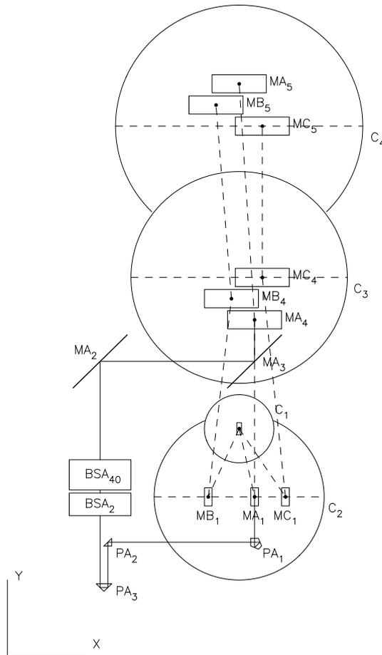
**Fig. 5.** Sketch of the optical design proposed for imaging spectro-polarimetry with EST/MSDP. The optical path between the first and the second spectrograph (from MA1 to MA4) is plotted for only one of the 3 lines A,B,C, recorded simultaneously.
