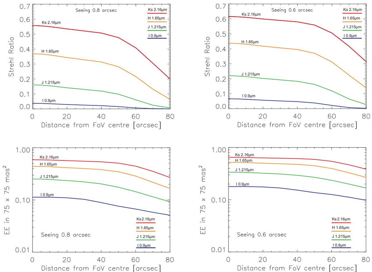
**Fig. 2.** MCAO module correction performance. Above: Strehl Ratio. Below: point spread function Ensquared Energy in  $75 \times 75 \text{ mas}^2$ . Left: seeing FWHM 0.8 arcsec. Right: seeing FWHM 0.6 arcsec.
