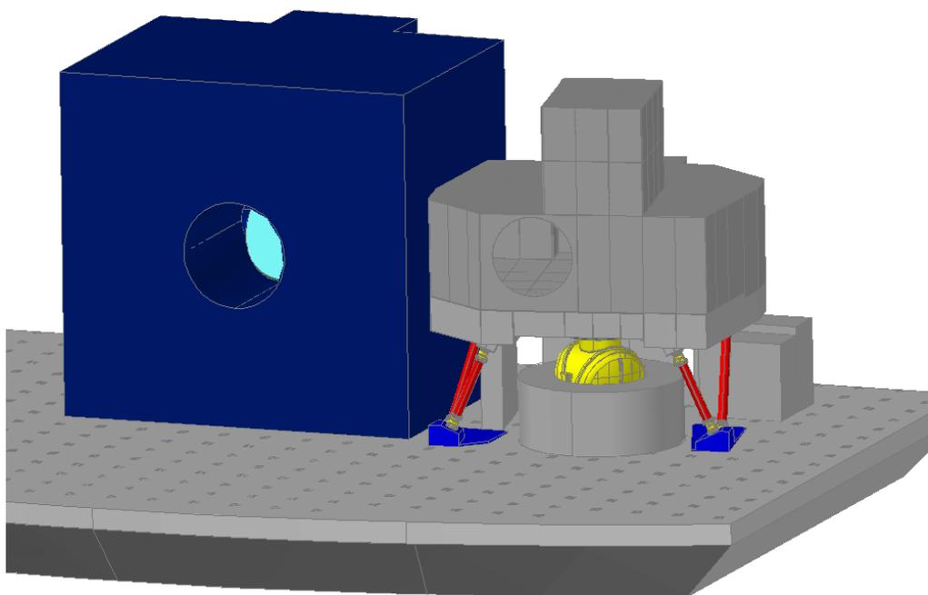
**Fig. 1.** Layout of MAORY on the E-ELT Nasmyth platform. The telescope pre-focal station is on the left part of the picture; MAORY is on the right. MICADO is shown underneath the optical bench of MAORY.
