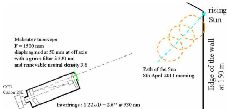
**Fig. 2.** Schematic of the experiment using a Maksutov imaging telescope, situated at 150 m from the edge of the wall when the rising Sun limb begins to appear
