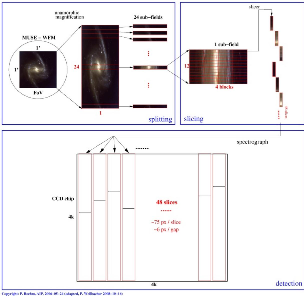
**Fig. 1.** Splitting of MUSE data: example given for the case of the Wide-Field Mode (WFM). The field splitter separates the  $1' \times 1'$  field-of-view into 24 sub-fields (**top-left**), each entering a separate IFU and sliced into 48 pseudo-slits (**top-right**). The various spectra produced are imaged onto a  $4k \times 4k$  detector (**bottom**). (Adapted from Weilbacher et al. 2009).
