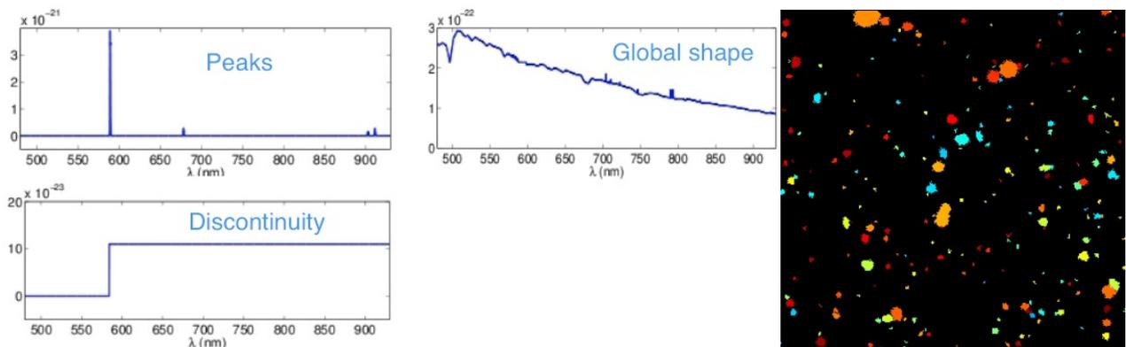
**Fig. 3. Left:** Example of “dictionary” of spectral shapes used in the segmentation technique: a given source spectrum is fitted by the linear combination of such shapes. **Right:** Example of datacube segmentation: sources are colored according to their spectrum.
