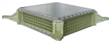
Fig. 2. The Electromagnetic Calorimeter honeycomb structure, before the final integration. PMTs are installed on the squared holes.
