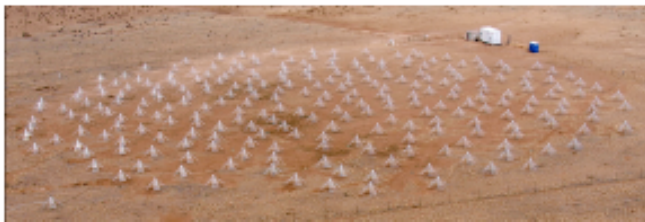
LWA & OLWA (USA) : 256 antennas, \varnothing=100 m, 10-88 MHz, beam former and imager in 8-16 MHz bandwidth (+ waveform snapshots)
