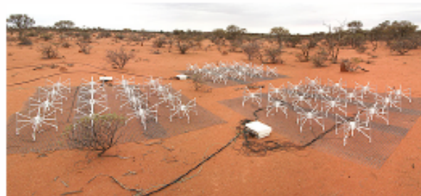
MWA (Australia) : 2048 antennas (128 tiles), \varnothing=3 km, 80-300 MHz, imager in 30 MHz bandwidth
