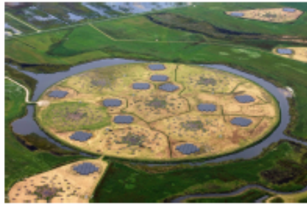
AARTFAAC (NL) : correlation of the 288 individual antennas of the LOFAR superterp, \varnothing=300 m, all-sky imager
